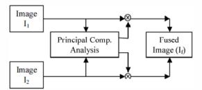
Figure 3: Image Fusion using PCA
